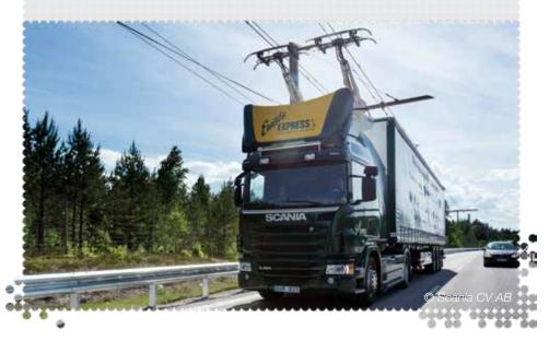
**132**: Siemens (April 2017) eHighway: solution for electrified road freight transport
